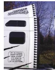
Rounding the vertical corners on the front and rear of the cab reduced drag by 40 percent while decreasing internal volume by only 1.3 percent. Likewise, rounding the vertical and horizontal corners cut drag by 54
